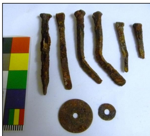
Plate 22. Nails pulled from the rotten bearers before disposal of the bearers (items 30).
